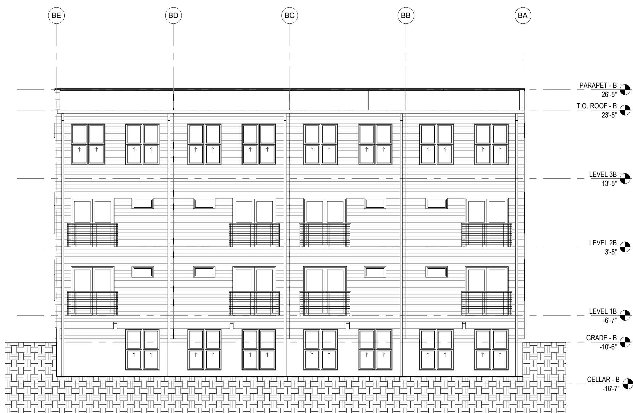
BUILDING B - NORTH ELEVATION 2 1/8" = 1'-0" A401
